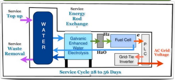
Service every 28 days or longer depending on installation power demands. Two hour service includes quick change electrodes, waste water removal and water top up. Hydrogen consumed within the fuel cell converts back to water to fuel G.E.E. hydrogen generator.
